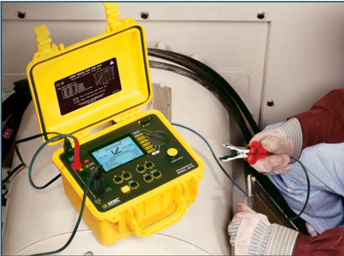
Model 5070 performing insulation test on a generator.
