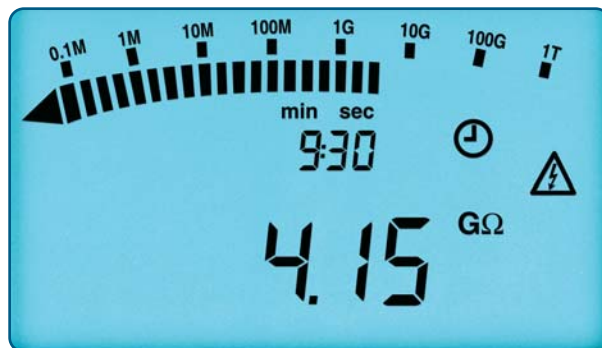
Automatic calculation and display of DAR ratio
