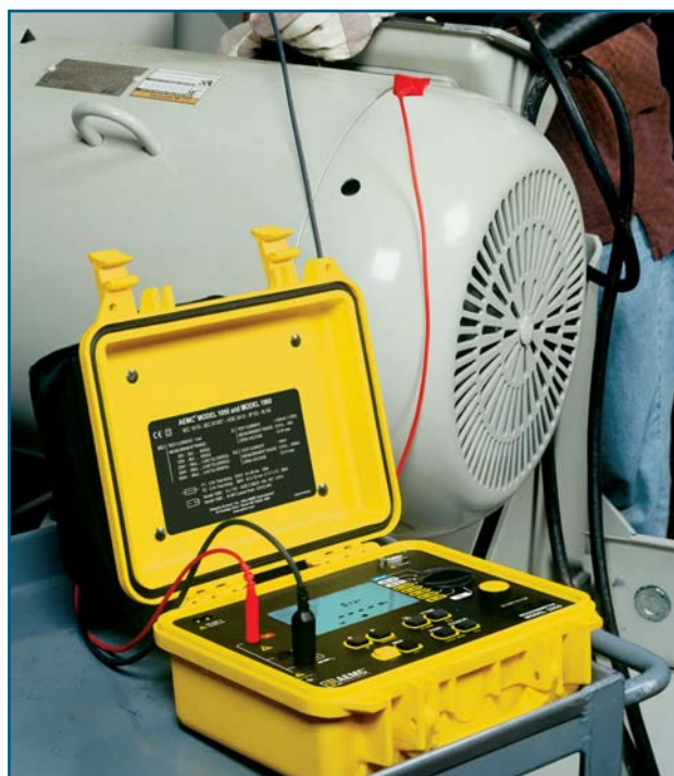
Model 1060 checking insulation resistance between windings on a three-phase motor.
